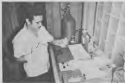
Lab Assistant Juan Vrolijk checks for the presence of oil in boiler water using the infra-red spectrophotometer.
